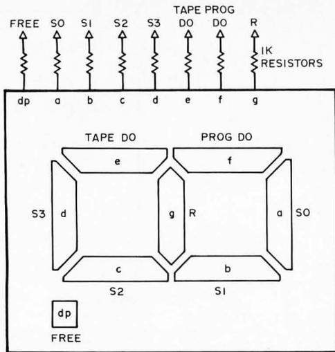
Figure 8: A 7 segment display is a compact way to provide all essential information for control and readout purposes.  $S_0$ – $S_3$  are the four bits of the counter  $S$ . The decimal point is available for other use, such as a logic probe function.
