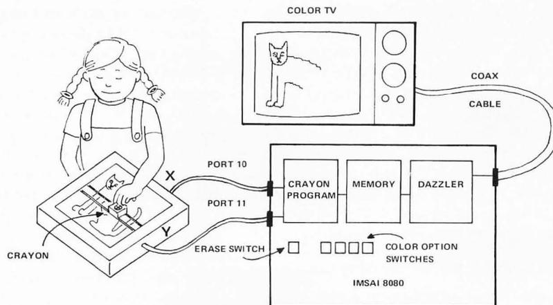
Figure 1: The Cybernetic Crayon System. The XY digitizer position is set by the young artist, and interpreted by the 8080 processor running a program shown in Listing 1. This program uses the position information along with the settings of front panel switches to determine the color value of each position in the picture as it is drawn.
