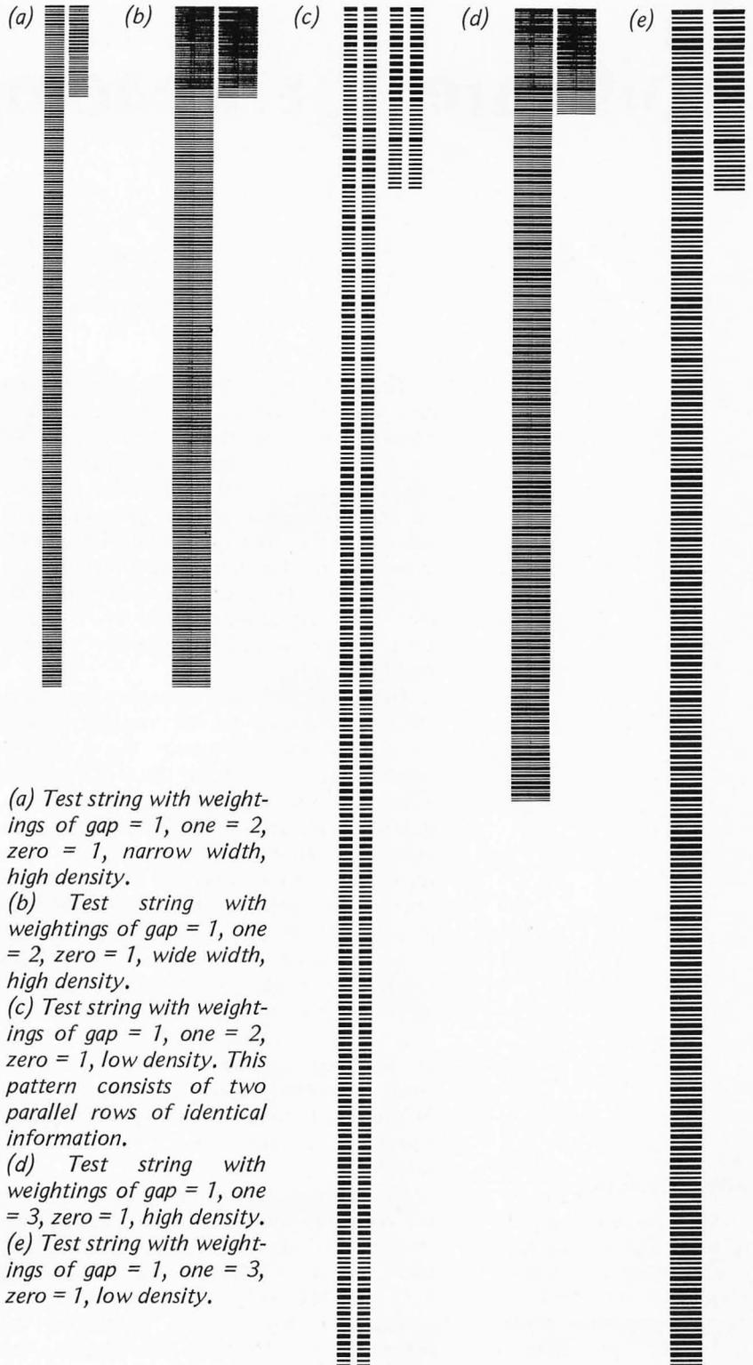
(a) Test string with weightings of gap = 1, one = 2, zero = 1, narrow width, high density.
