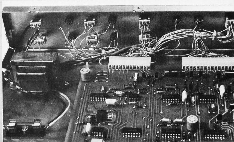
Figure 1: Modulator and Demodulator Circuitry of the AC-30. This diagram shows the portion of the AC-30 used to create the output signal, and decode the two frequencies on input. All interfaces to the user system are via the control logic of figure 2. Power connections for integrated circuits are found in table 1.
