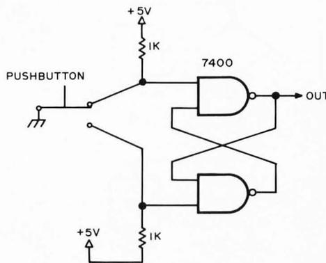
Figure 7: Debouncing circuit for an SPDT push button.
