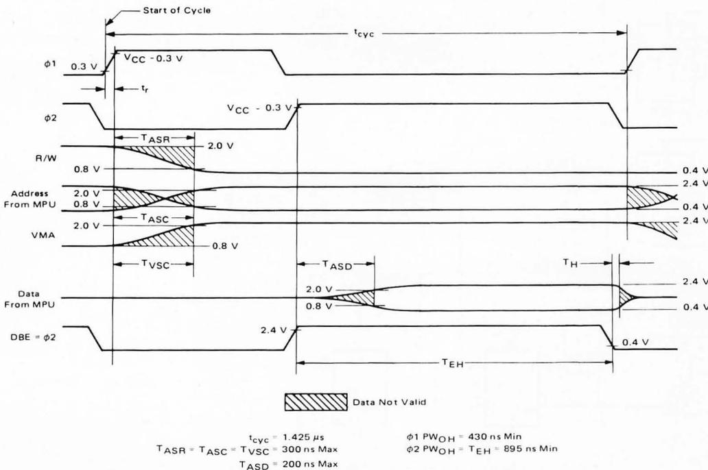
Figure 2b: Nominal Memory or Peripheral Write Cycle, stretched by holding the  $\Phi_2$  state to accommodate a slow memory circuit. This diagram is reproduced courtesy of Motorola Semiconductor Products Inc, from page 4-53 of the M6800 Microprocessor Applications Manual.
