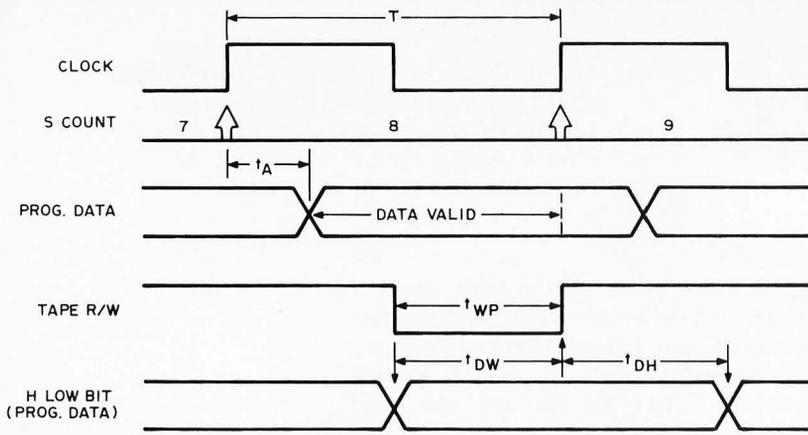
Figure 4: The *w* bit of an instruction is read from the program 2102 and written into the tape 2102 with the sequence of events shown in this timing diagram. The *w* data is shifted into H so that it will be steady during the data setup ( $t_{DW}$ ) and data hold ( $t_{DH}$ ) intervals. The clock half cycle must be longer than  $t_A$ , which is  $1 \mu s$  for a slow 2102.
