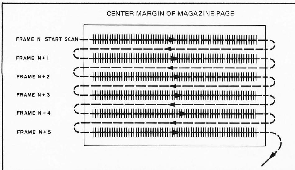
Figure 3: Page Layout. A page of data in printed form [as we would run in BYTE] would be laid out with the data running parallel to the center margin of the magazine. This allows the maximum amount of data in a frame, thus minimizing the overhead bits of the frame format.
