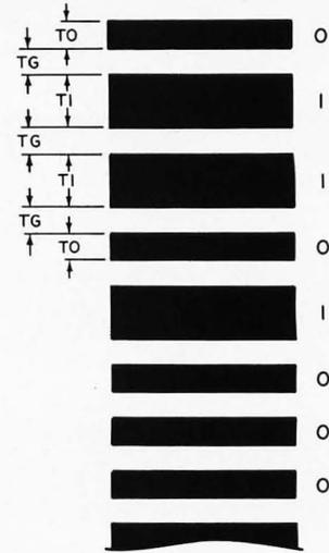
Figure 1c: Format 3: Fixed gap bar width modulation. The parameters to be specified in printing are the interbar gap width  $T_G$ , and the bit length parameters  $T_0$  and  $T_1$ . In reading this code, the length of the interbit gap gives a calibration for judging the next dark period as a 0 bit (short) or 1 bit (long). The data density (as in format 1) varies with the statistics of the number of 0s and 1s in a given region of the printed data.
