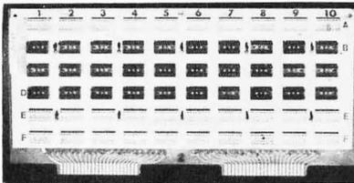
These are prototype boards that can be used in almost any type of wirewrap application. The board consists of a (top) positive plane and the other side is a negative plane. There are two 44 pin connectors that may be utilized. There are 30 16 pin sockets and 30 14 pin sockets. All these pins are gold plated. The wire wrapping that is in the back can very easily be removed. We have a limited quantity of these boards. so act quickly.
