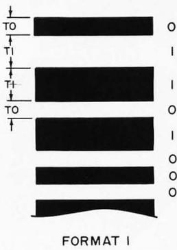
Figure 1a: Format 1: Bar width modulation, with alternate dark and light. The parameters to be specified in printing are widths  $T_0$  and  $T_1$ . A trailing bit complementary to the last data bit in a string is required. The leading bit of a string will be assumed to be in the dark state. In reading this code, time between transitions falls into two categories, long for a 1 bit, and short for a 0 bit.
