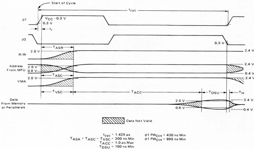
Figure 2a: Nominal Memory or Peripheral Read Cycle, stretched by holding the  $\Phi_2$  state to accommodate slow memory circuits. This diagram is reproduced courtesy of Motorola Semiconductor Products Inc, from page 4-52 of the M6800 Microprocessor Applications Manual. In the SWTPC system modification described, the actual timing values are scaled to its clock speed, but the idea is the same.
