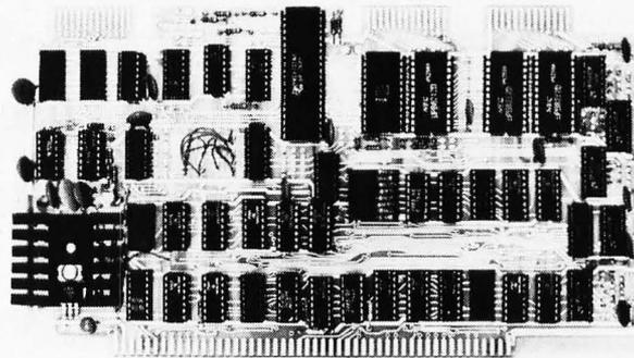
**IMSAI MULTIPLE I/O BOARD.** Simultaneous control of keyboard, printer, tape cassette (Byte or Tarbell) and teletype (or CRT) by a single MIO board. Our 5-port, multiple I/O board combines the most commonly used I/O interfaces including a cassette interface, two parallel I/O ports, one serial channel and one control port—all on one board!
