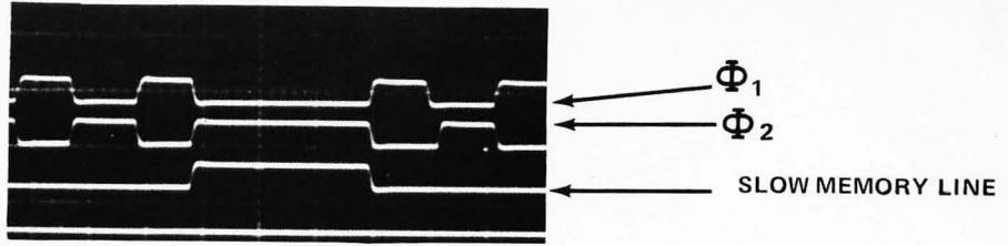
Photo 1: This is an oscilloscope camera tracing of the slow memory interface timing resulting from the author's circuit. The upper traces are  $\Phi_1$  and  $\Phi_2$  (see markings). The lower trace shows the slow memory line, which stretches the  $\Phi_2$  out for one full clock cycle of extra time.
